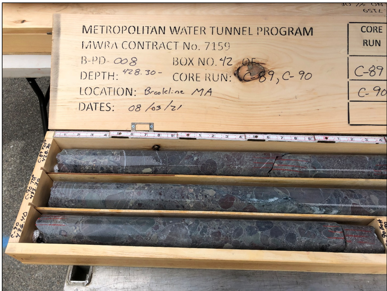
Figure 2. Typical Rock Cores Extracted from a Boring.
